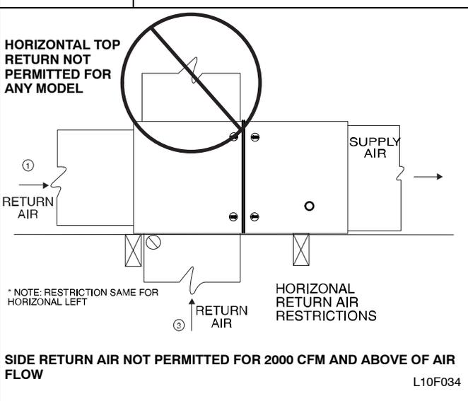
SIDE RETURN AIR NOT PERMITTED FOR 2000 CFM AND ABOVE OF AIR FLOW
