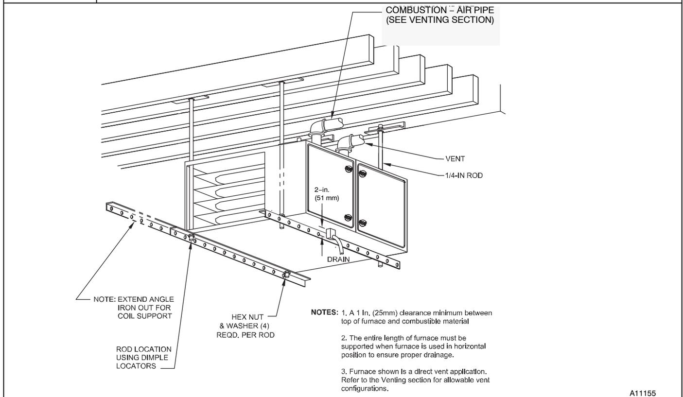
**NOTE: Local codes may require a drain pan and condensate trap when a condensing furnace is installed over a finished ceiling**
