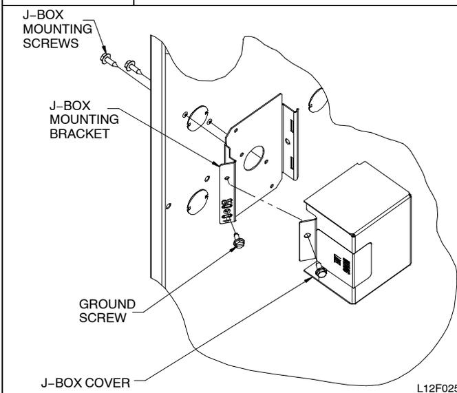
5. Route external field power wires through holes in electrical box and casing.
