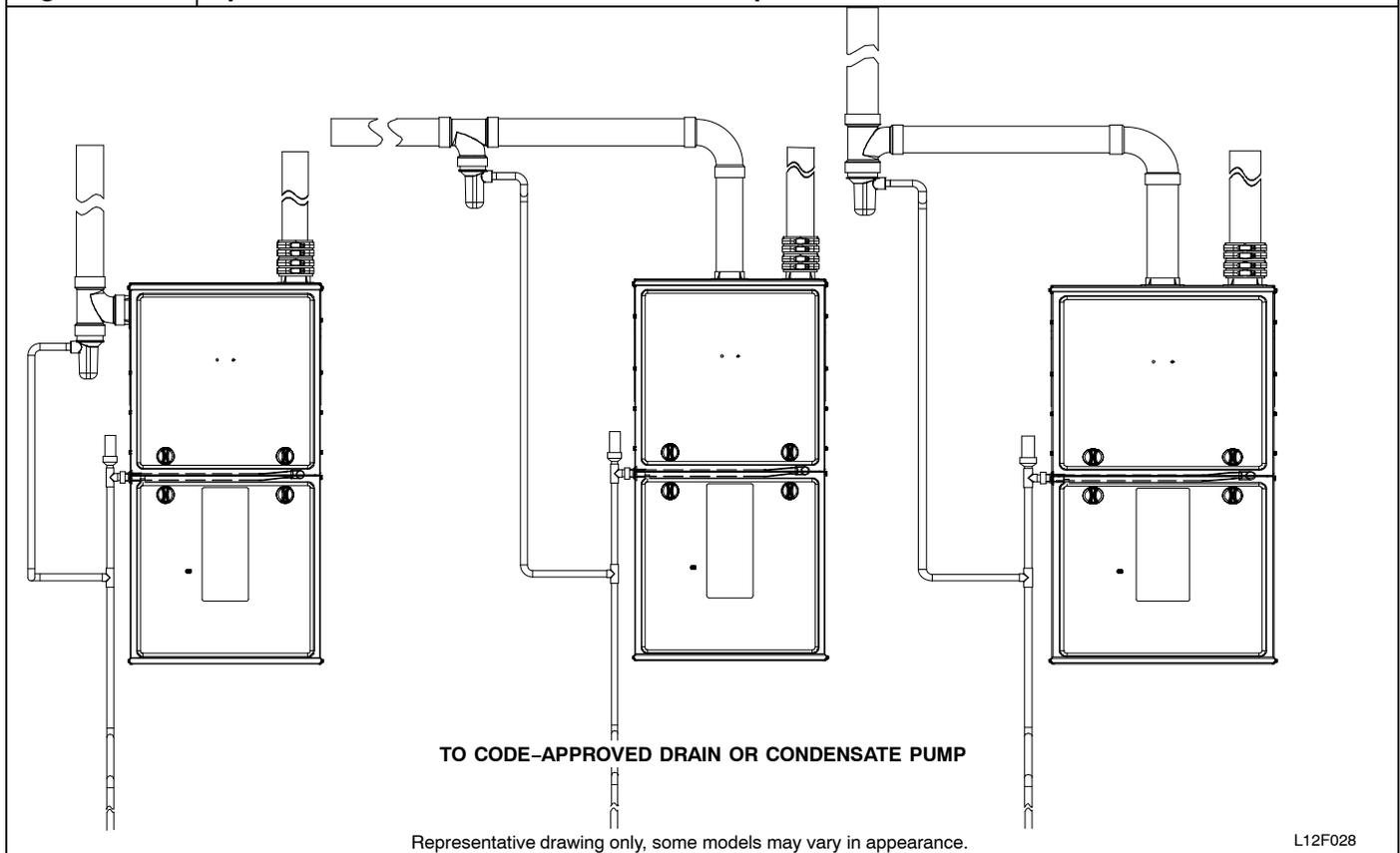
The External Vent Trap Kit accessory may be used as a trap for the combustion air inlet pipe if a large amount of moisture must be removed. The drain line may be connected to the same drain as the furnace condensate and the evaporator coil condensate line **ONLY** if the inlet air trap drain and the evaporator coil drain empty into an open segment of pipe above the drain, See **Figure 12**. When using the External Vent Trap Kit, refer to those instructions for proper drain connections.
