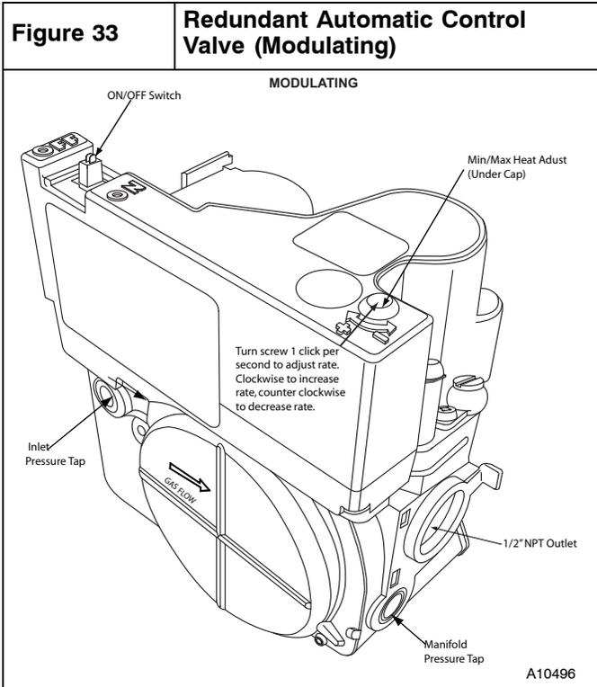
If pressure exceeds 0.5 psig (14-in. w.c.), gas supply pipe must be disconnected from furnace and capped before and during supply pipe pressure test. If test pressure is equal to or less than 0.5 psig (14-in. w.c.), turn off electric shutoff switch located on furnace gas control valve and accessible manual equipment shutoff valve before and during supply pipe pressure test. After all connections have been made, purge lines and check for leakage at furnace prior to operating furnace.
