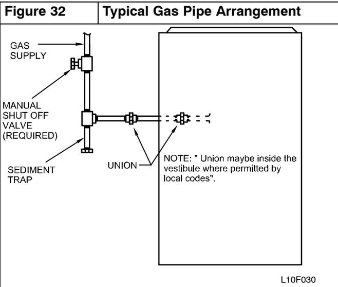
A 1/8-in. (3 mm) NPT plugged tapping, accessible for test gauge connection, **MUST** be installed immediately upstream of gas supply connection to furnace and downstream of manual equipment shutoff valve.
